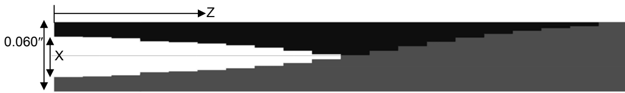
Figure 3a: Matching transformer section of the balun showing the offset.
